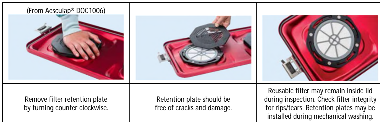
Figure 3: PrimeLine™ Pro Lid Inspection Process
