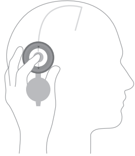
Fig. 9: Localizing the valve using the M.blue Compass
